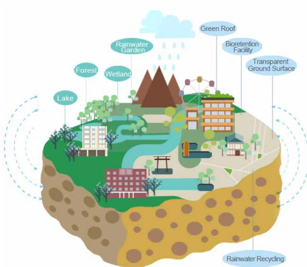
A "Sponge city" refers to a city where its urban underground water system operates like a sponge to absorb, store, leak and purify rainwater, and release it for reuse when necessary.
